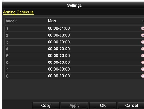
Figure 8-17 Set Arming Schedule of Alarm Output
