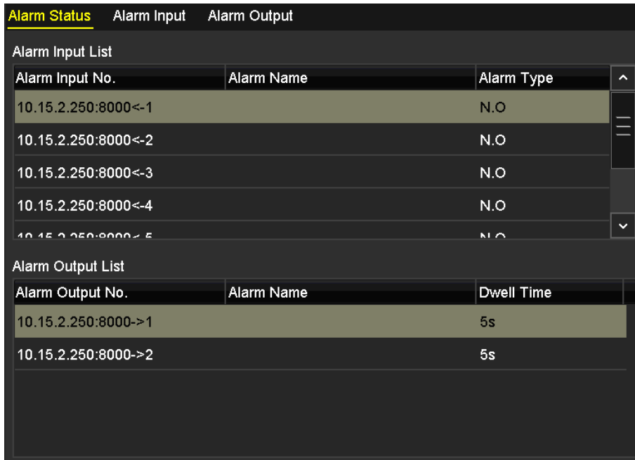
Figure 8-4 Alarm Status Interface of System Configuration
